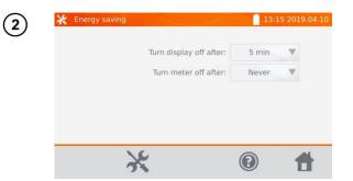
Set the inactivity time for blanking the screen and turning the meter off.
